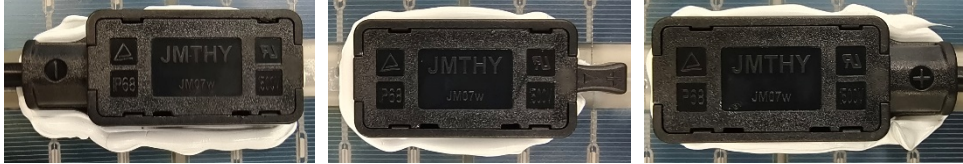
Fig. 3: View of junction box of module type Eagle-66HCB690M
